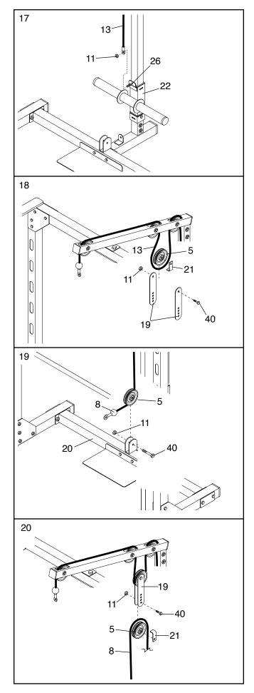
Attach the indicated end of the Low Cable (8) to the bracket on the Rear Base (3) using an M10 x 20mm Bolt (26) and an M10 Nylon Locknut (11).
